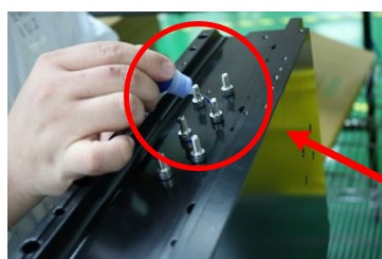
Fig. 5.15: Use non-magnetic tool to install the stator
