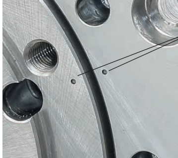
Fig. 5.5 Index marking for position encoder
