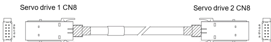
Fig. 16.14: Servo drive communication cable (for gantry control system)
