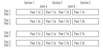
For paired multi-part rails, the butt joints should be staggered.
