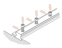
5) Tighten rail mounting bolts in three stages using a torque wrench until the specified torque is reached
