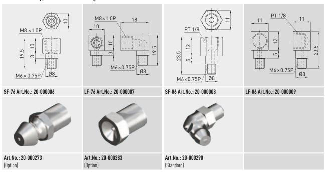
Table 4.5 Grease nipples and lubrication fittings 1/8 PT
