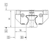
Table 3.57 Tolerance of parallelism between block and rail
