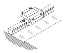
4) Tighten clamping screws one after another in order to ensure good contact between the rail and the reference edge
