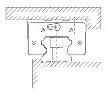
Profile rails that are not attached to an installation surface may have larger tolerances in terms of straightness. Below you will find typical mounting situations: Details of the assembly tolerances can be found in the chapters for the individual series.
