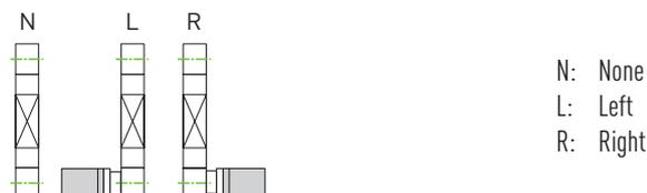
Fig. 4.13 Drive interfaces of the linear axis HM-B
