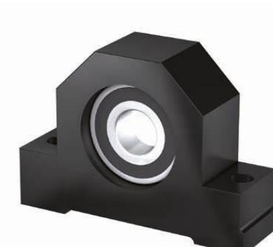
The axis height of the supported bearing is matched to fixed bearing SFA and nut housing GFD. The housing can be screwed on from above (S1) and below (S2). The reference edge makes it easier to align the unit. The end machining suited to the supported bearing is the S5-xx or S1-xx type.
